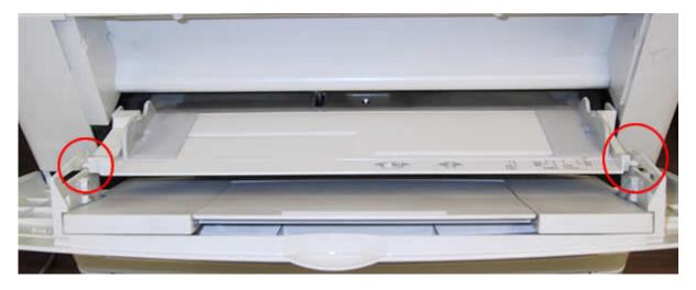
Flip the inner tray up and the outer tray will come off by sliding it to the right. Remove the inner tray by letting it rotate all of the way down. It should fall right out of its pivot/hinge.
