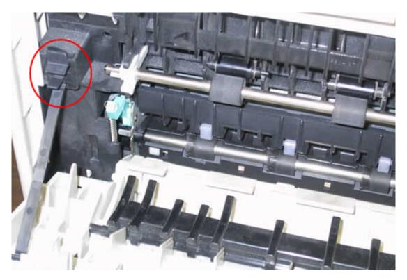
Slide the door to the left to remove it. Remember that when you re-install the door to insert the pin on the left side of the cover first.
