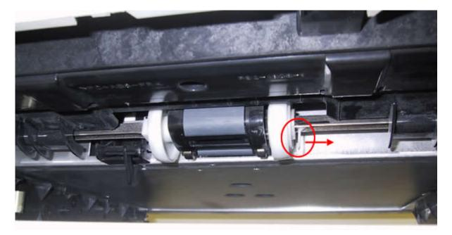
Slide the roller to the left so it is centered between the two white discs. Rotate the roller 180 degrees and it will drop down.
