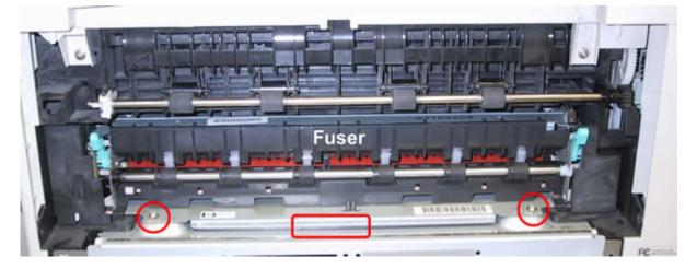
Install the replacement fuser in reverse order and reassemble the back cover.
