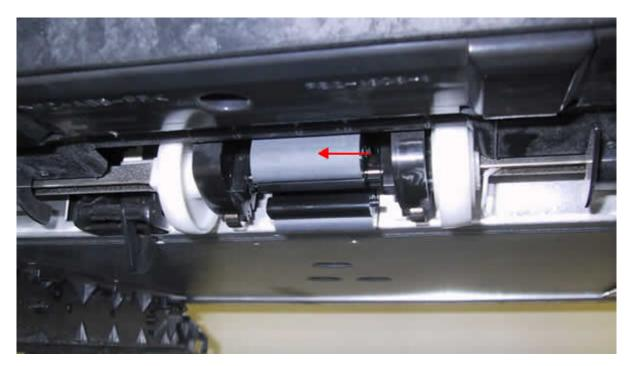
To install the replacement roller make sure the pin on the roller circled below is on the right. Rotate the roller 180 degrees so the rubber is facing up. Slide the white disc toward the center and make sure the roller is seated.
