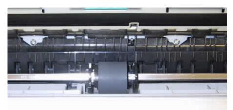
Before replacing the transfer roller, replace the separation pad.
