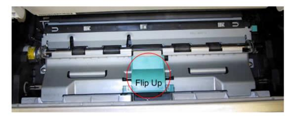
Squeeze the pick-up roller and slide it to the right.
