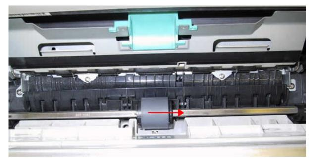
The roller is sandwiched between two black discs. Slide the roller back to the left so it is centered between the discs and pull the roller straight up and out.
