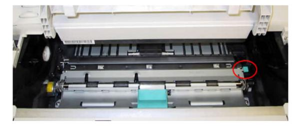
Remove the two screws circled below and remove the metal plate.
