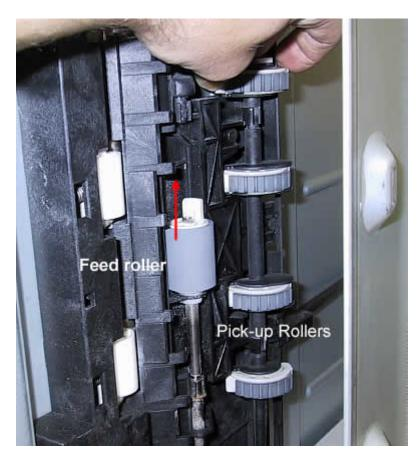
Now replace the pickup rollers. Remove them by pressing on the locking tab circled below, rotate the shaft, and pull
