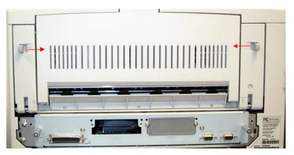
Pinch the plastic support strap located on the left side. Squeeze the tab while pulling up to remove the support strap. This will take a little wiggling and tugging to get the strap out.
