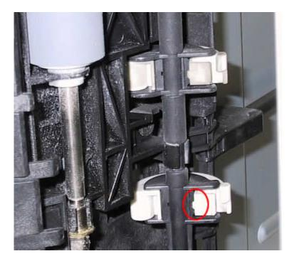
The separation roller in the paper tray is replaced by opening the hinged door and pulling the roller off of the shaft.
