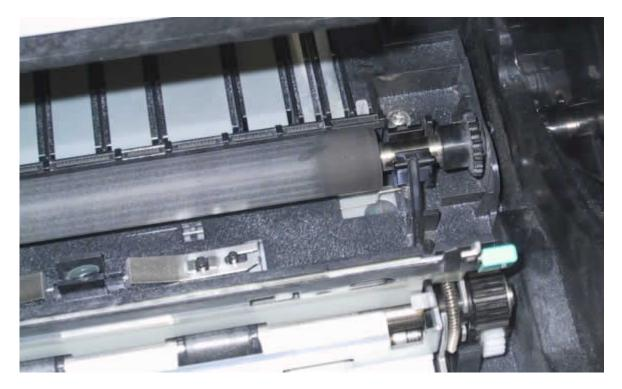
Use the small blue plastic transfer roller removal tool that came with your printer to pry up the left side of the transfer roller. Then remove the right side of the roller from its mount.
