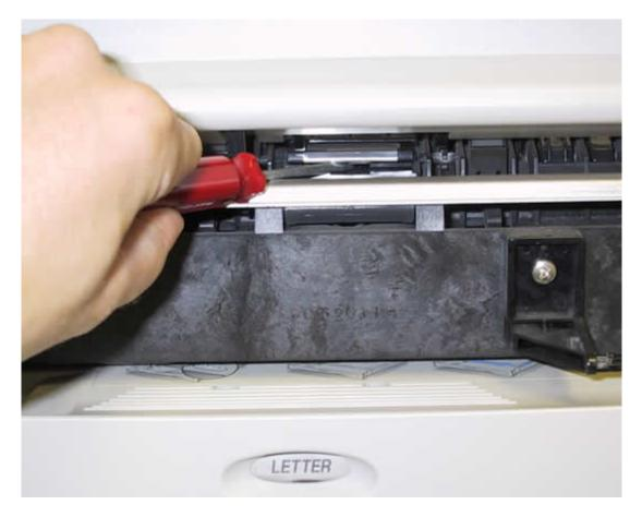
Install the new pick-up roller by making sure the thumb grip is on the left. You can only install the roller one way. Slide the roller to the right until it is seated against the right black plastic disc. You might have to slightly lift and wiggle the roller to get it seated. Now slide the right disc and the roller all of the way to the left until it clicks into place.
